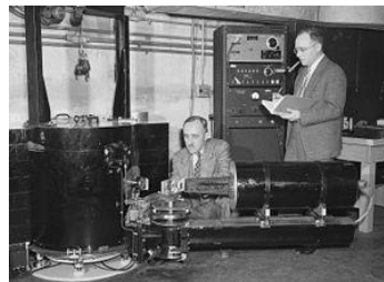
Clifford Shull (right) working with a double-crystal neutron spectrometer
